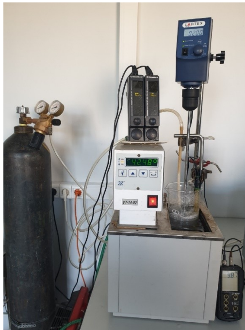
Figure 4. Laboratory setup for carbonation of pond liquor at different temperatures.
